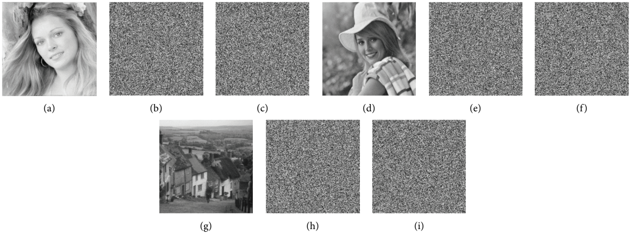
FIGURE 11: Recovered images using a slightly changed key. (a) Face. (b) Encrypted face. (c) Decrypted face. (d) Elaine. (e) Decrypted Elaine. (f) Decrypted Elaine. (g) Hill. (h) Encrypted hill. (i) Decrypted hill.
