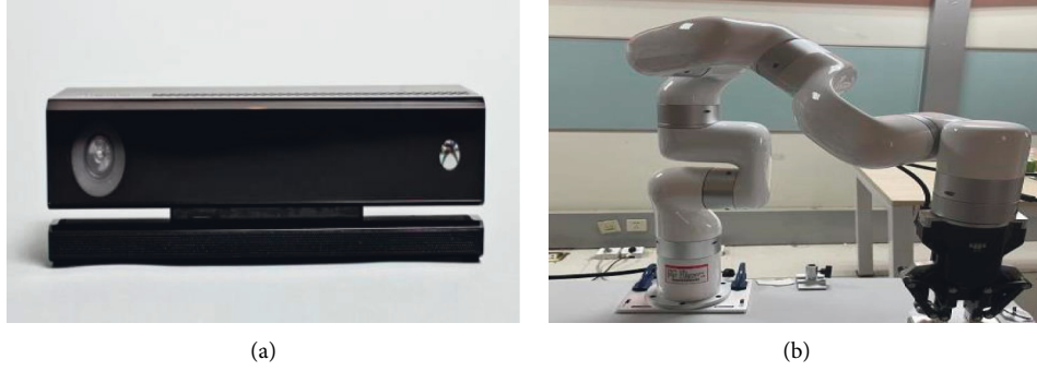
FIGURE 1: Interactive device diagram for intelligent massage positioning systems: (a) Kinect 2.0 devices; (b) xArm robotic arm devices.
