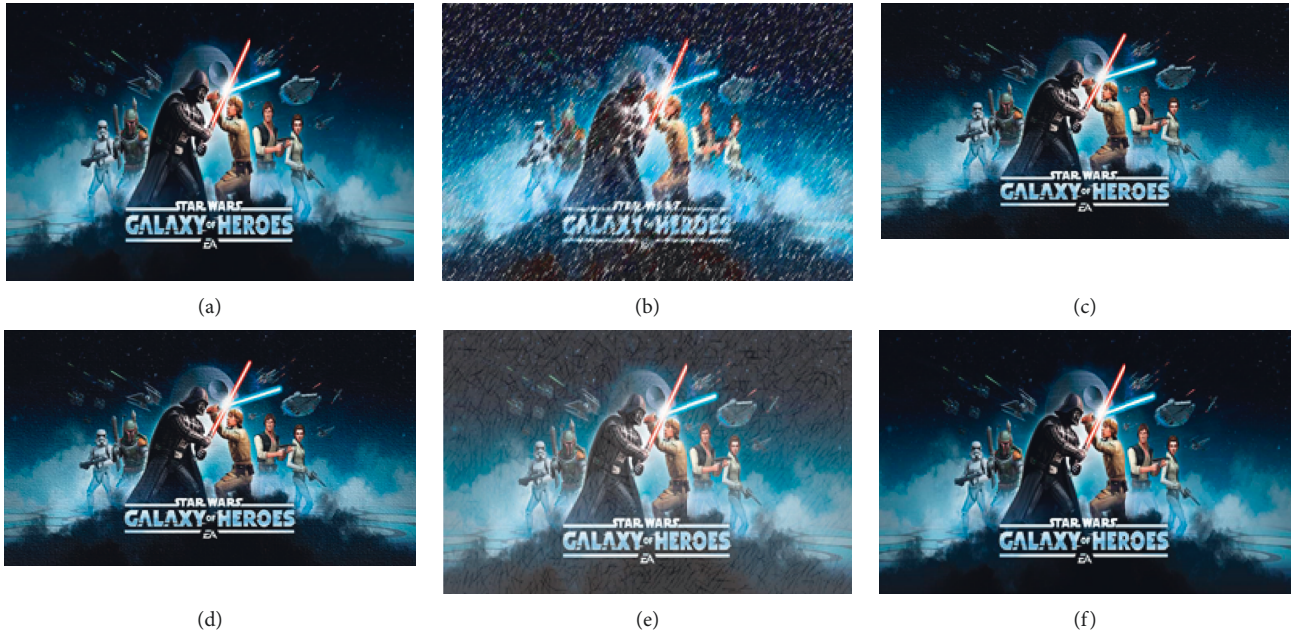
FIGURE 8: Comparison of the image optimization effects of different methods: (a) original image; (b) image after adding salt and pepper noise; (c) simulation system; (d) FPGA; (e) DSP; (f) the algorithm proposed here.
