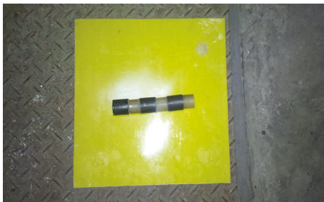
FIGURE 6: Phononic crystal is composed of steel and silicone rubber.
