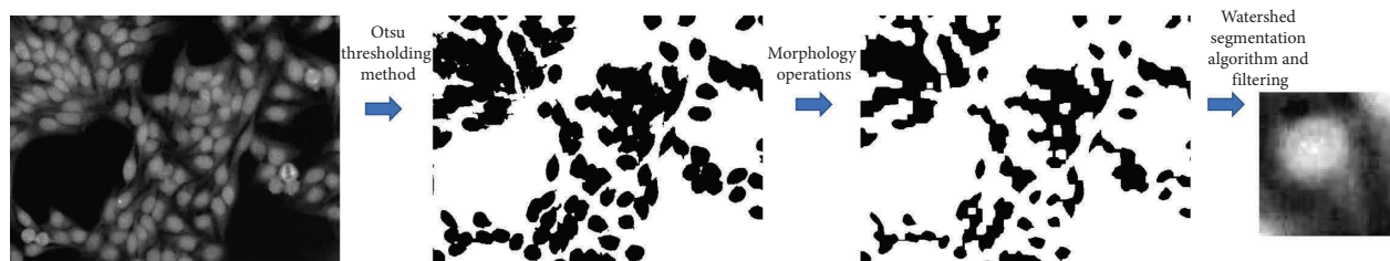
FIGURE 5: Process of using Otsu thresholding method and watershed segmentation algorithm.
