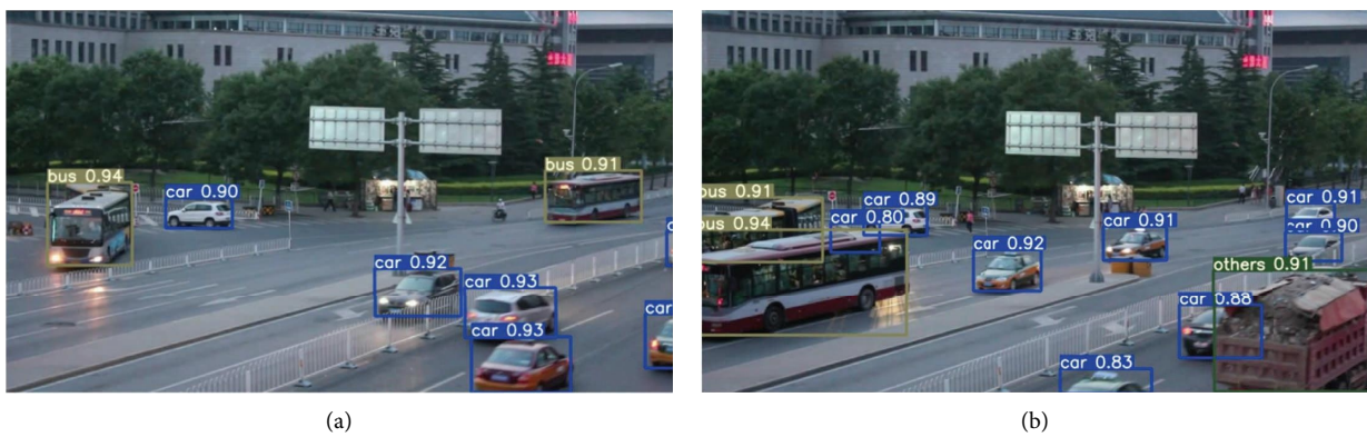
FIGURE 12: YOLOv5s_DSC vehicle detection at the oblique side of the intersection.
