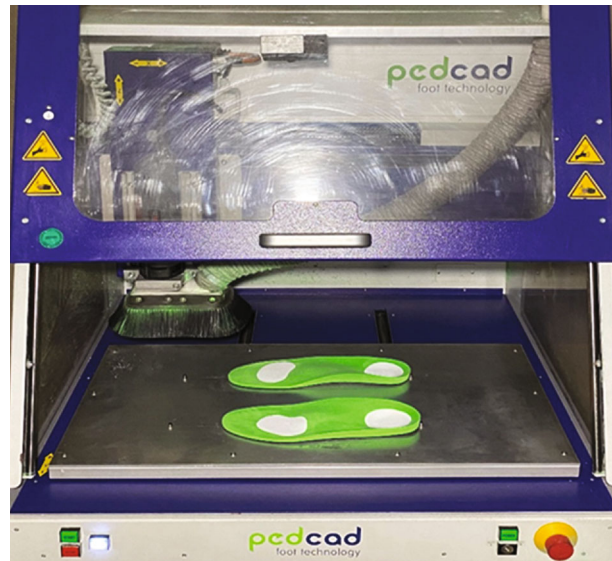
FIGURE 8: The individual orthopedic insoles, taking into account the locally over-pressured areas on the plantar side of the foot.
