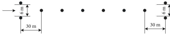
FIGURE 21: Overview of snake testing.
