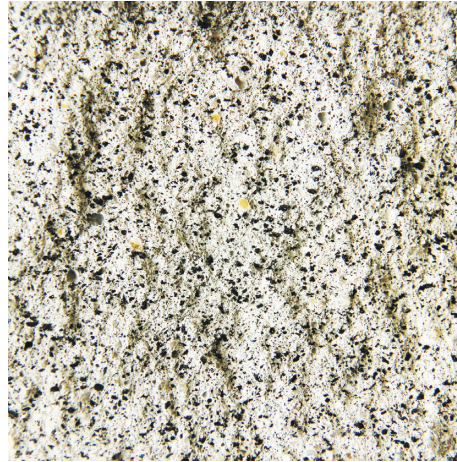
FIGURE 16: Profile map of K1 group with a uniformity of 1.16. The mixing amount of cellulose ether is 4.6351 kg and the substitution rate of rubber is 0.4268.
