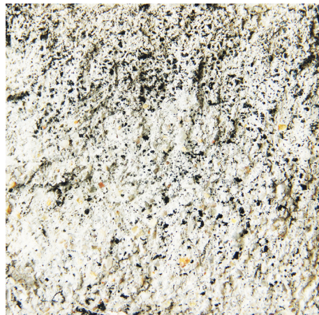
FIGURE 17: Profile map of K5 group with a uniformity of 0.32. The mixing amount of cellulose ether is 0 and the substitution rate of rubber is 0.25.
