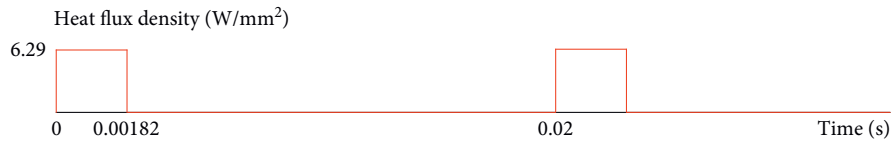
FIGURE 15: The loading process of the first load step of the driving gear.
