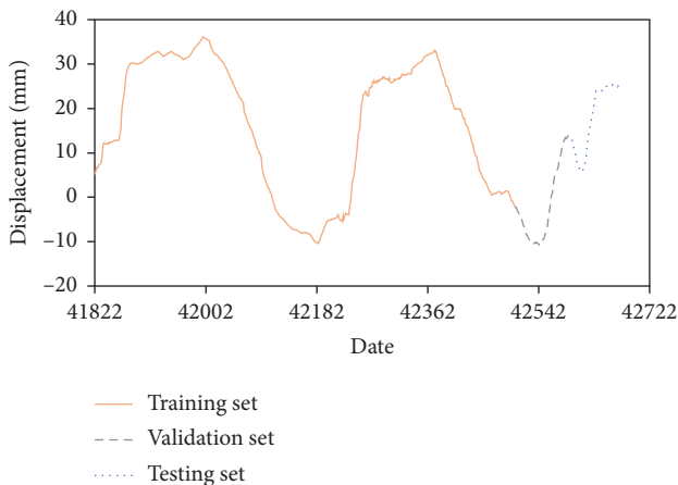
FIGURE 5: Displacement recorded by the pendulum at block 13.
