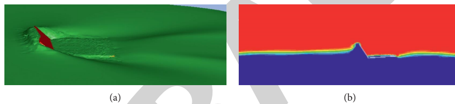
FIGURE 4: Simulation results of 50° floating plate. (a) 50° free waveform diagram. (b) 50° volume fraction diagram.
