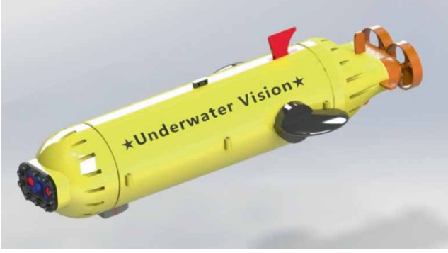
FIGURE 1: Three-dimensional model of UUV equipped with vision system.
