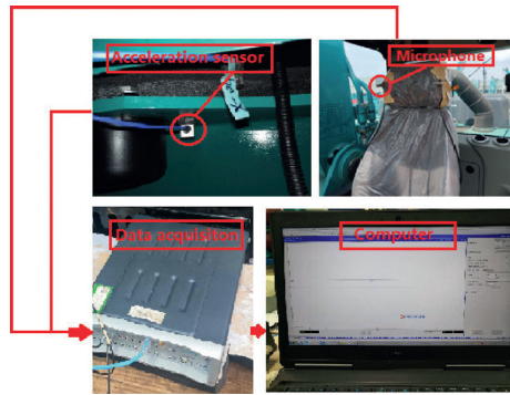
FIGURE 6: Baseline measurements for vibration and noise.
