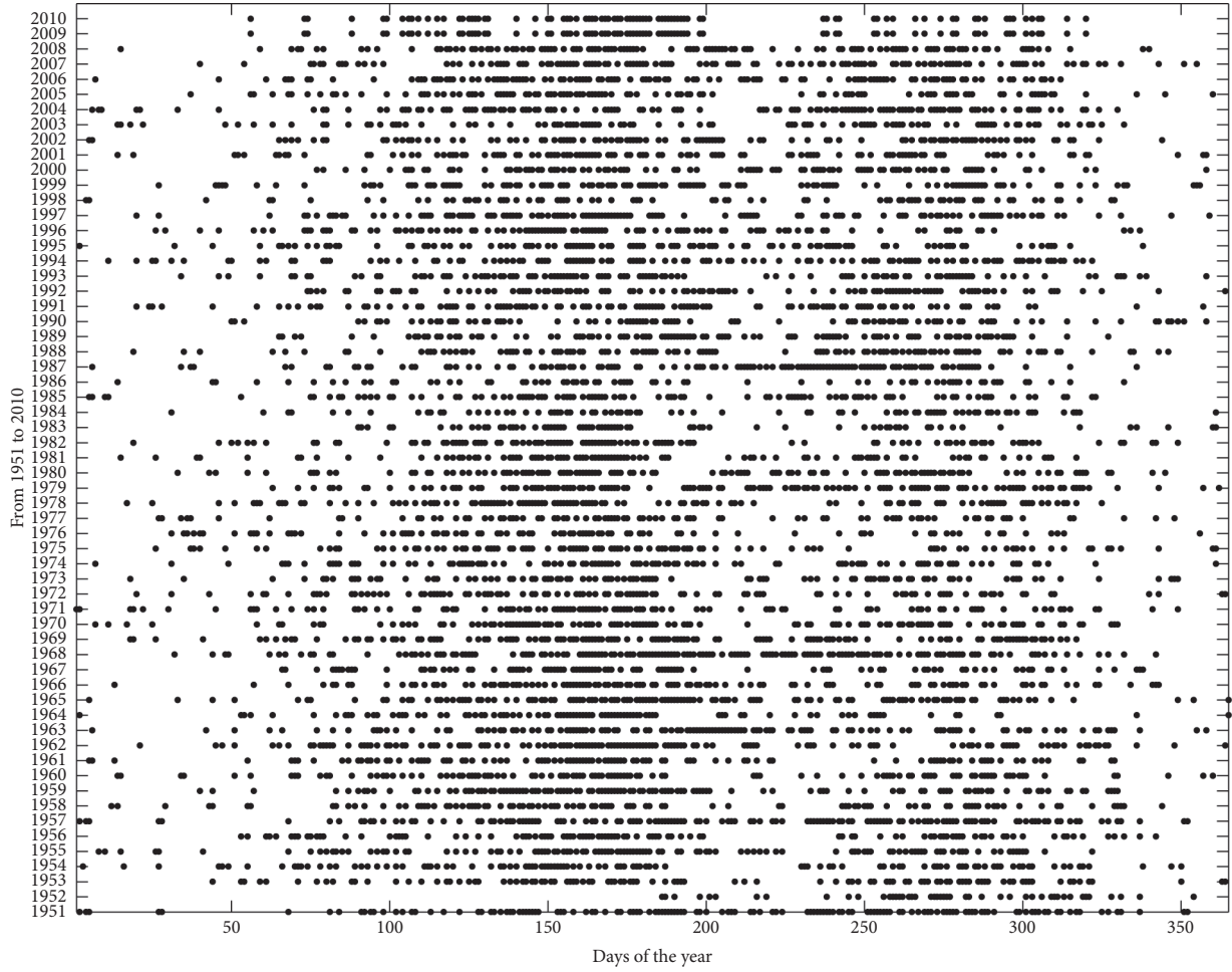
FIGURE 2: Daily rainfall occurrence during 60 years of observations in the Cotonou synoptic station. Each row corresponds to a year of observations. The occurrence of rain is defined by a precipitation threshold that distinguishes between dry and rainy days. The precipitation threshold chosen in this representation is zero.
