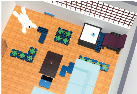
FIGURE 3: Operation of P-hTetro in a typical indoor environment. The robot shrinks its size in narrow spaces to improve the coverage. Similarly, the robot expands its size in free areas.
