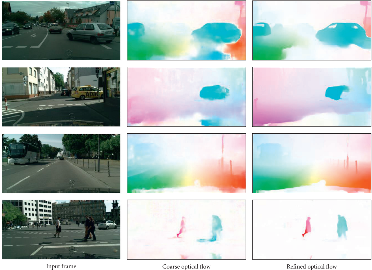
FIGURE 3: Visual comparison on the Cityscapes dataset for the original optical flow. The first column denotes the input frame. The middle column denotes the coarse optical flow produced by the optical flow network. The last column denotes the refined optical flow optimized by the flow refinement module. The refined optical flow has sharper motion boundaries than the original optical flow.
