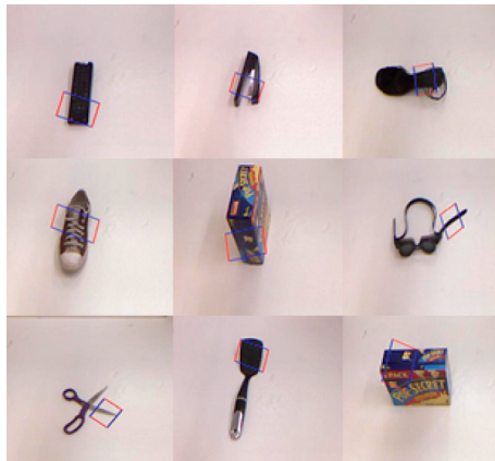
FIGURE 6: The results of grasp detection on several images of Cornell Grasp Dataset.
