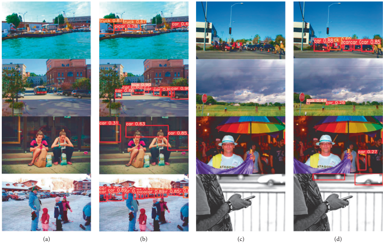
FIGURE 9: Examples of visualizations. (a, c) The original diagram contains the vehicle at various angles, far and near perspective, and even includes the reflective glass vehicle. (b, d) The result of the visualization of the improved model.
