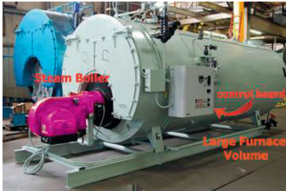
FIGURE 1: A power plant boiler.
