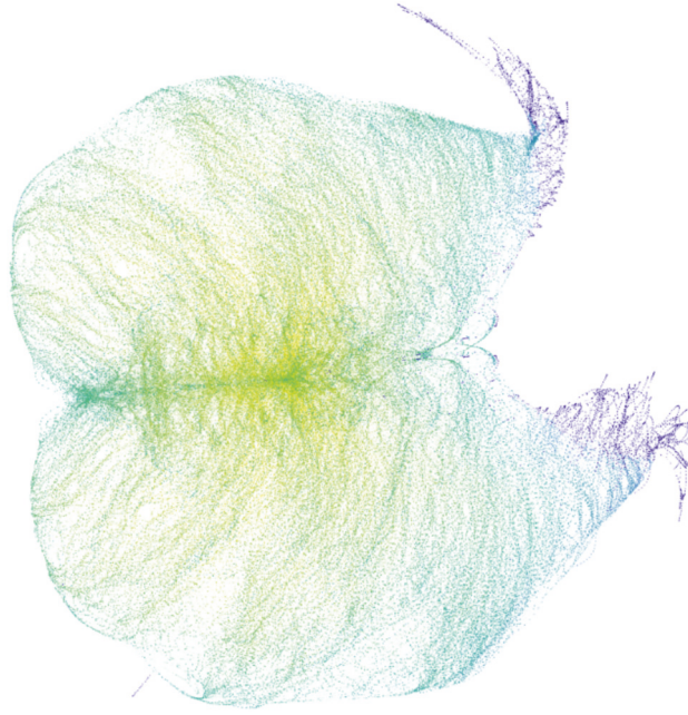
FIGURE 5: SSCC of the four-dimensional chaotic system as a network. Nodes colors are based on node attractivity from blue (low) to yellow (high).
