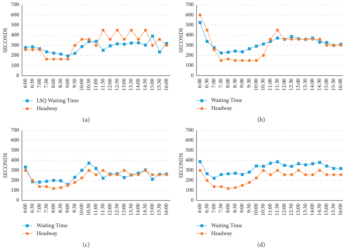
FIGURE 6: Average waiting time at transfer platforms.
