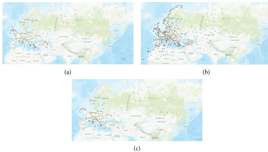
FIGURE 8: LCC of the Europe-Russia component after its isolation from the network. The black dots are the remaining airports after attacks on the world air transportation network (a) strength attack, (b) weighted betweenness attack, and (c) weighted PageRank attack. The LCC isolated by the strength and weighted PageRank attacks covers almost all countries sparsely. The LCC is well distributed in all the initial component areas for the weighted betweenness attack.
