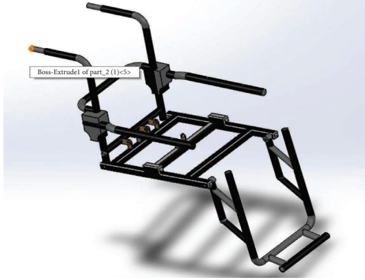
FIGURE 3: Frame assembly in SolidWorks.
