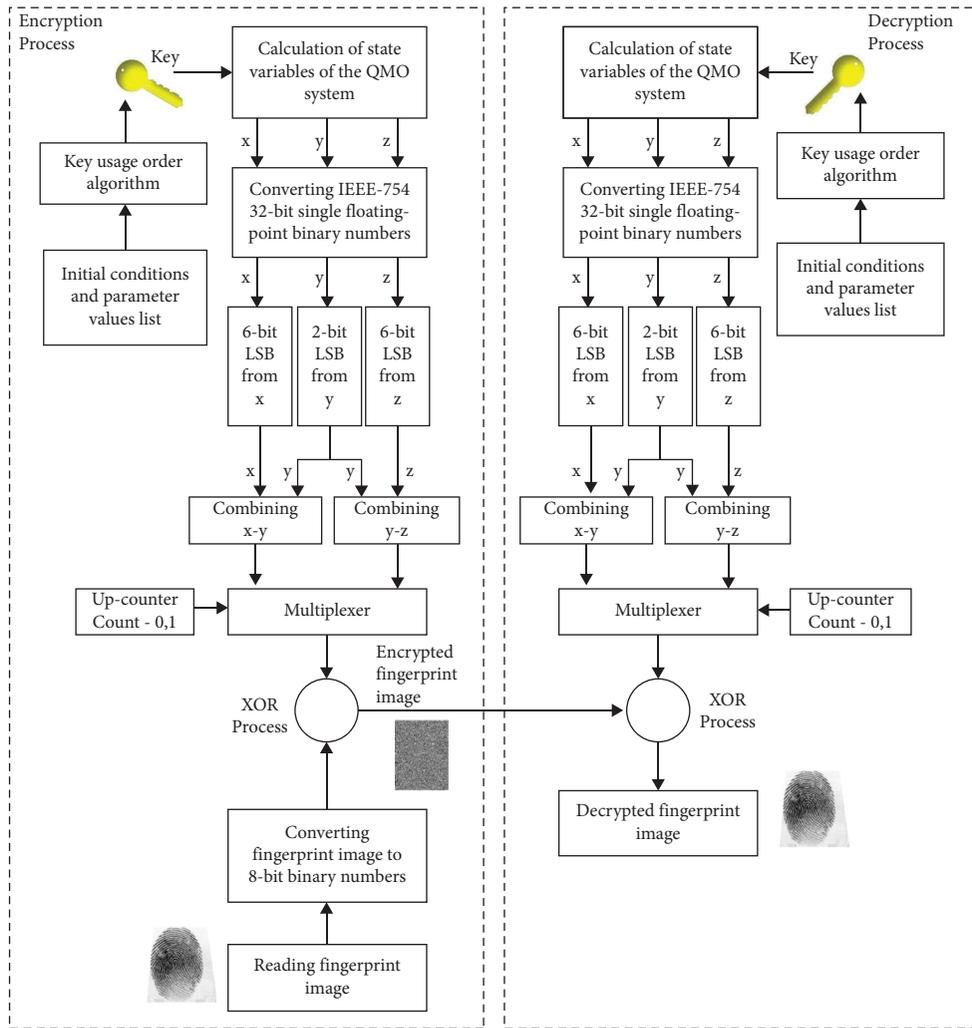
FIGURE 5: The encryption and decryption processes diagram.
