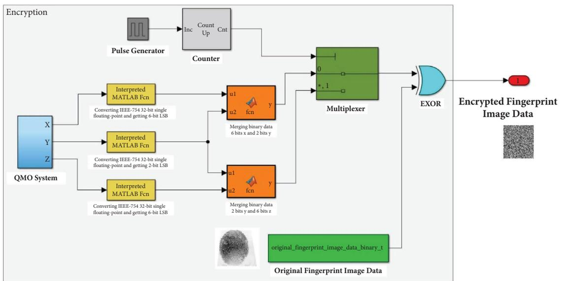
FIGURE 6: Simulink diagram of the encryption process.
