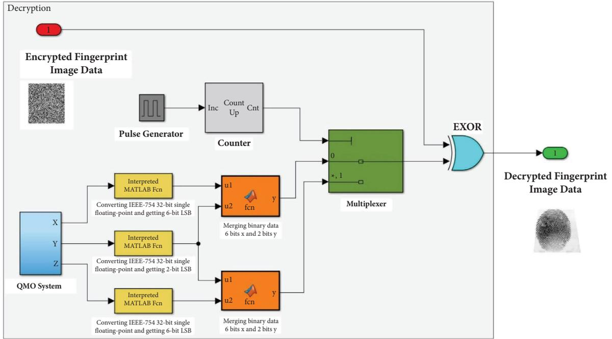
FIGURE 7: Simulink diagram of the decryption process.
