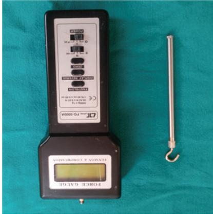
FIGURE 8: Digital force measurement gauge.
