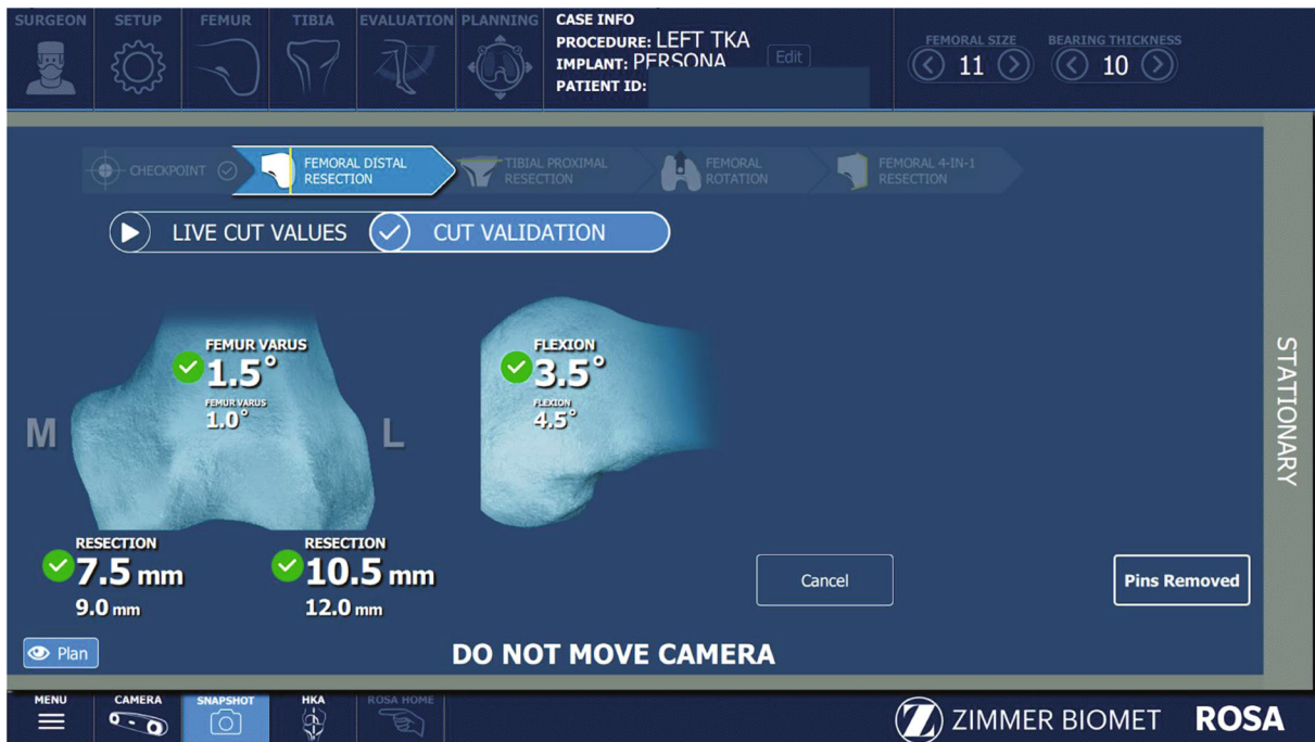
FIGURE 10: Final distal femoral resections validated against planned resections for Case 3.
