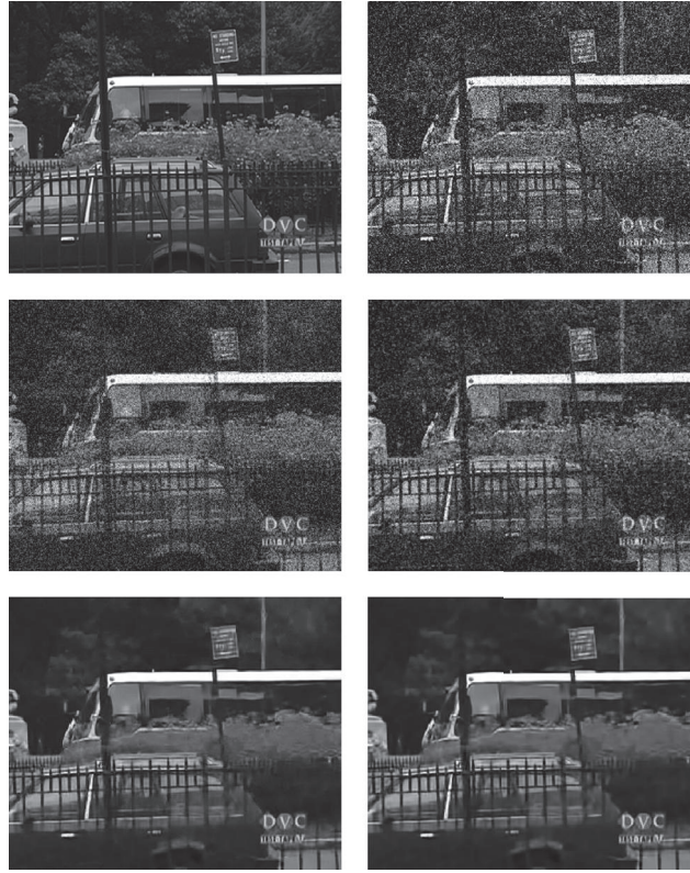
FIGURE 4: Visual comparison of different algorithms for frame 5 of Bus sequence. From left to right and from top to bottom: original frame, noisy frame ( \sigma_n = 40 ), result of [18] algorithm, result of [19] algorithm, result of [13] algorithm, and result of the proposed algorithm.
