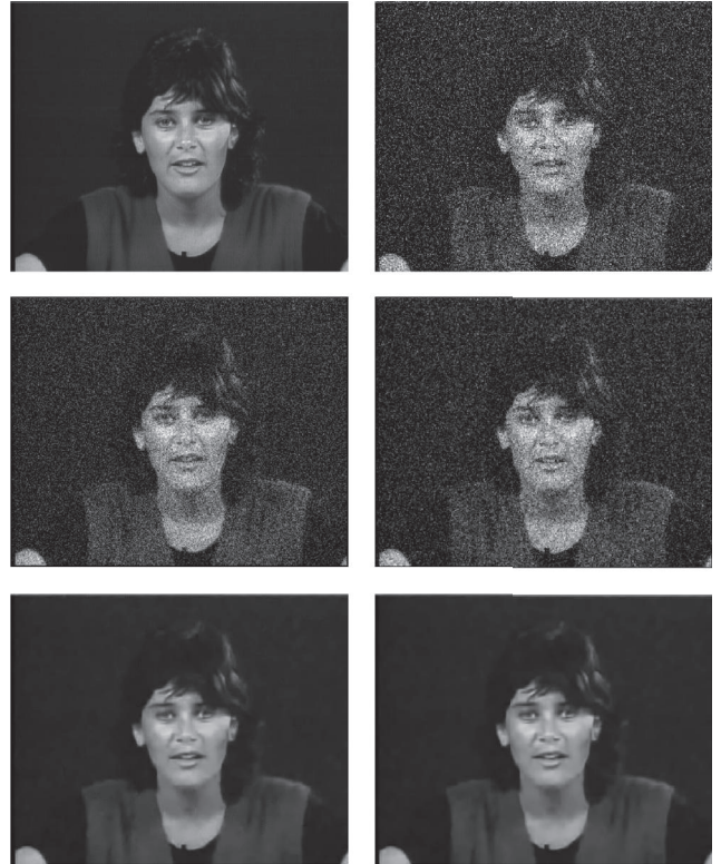
FIGURE 1: Visual comparison of different algorithms for frame 5 of the Miss America sequence. From left to right and from top to bottom: original frame, noisy frame ( \sigma_n = 40 ), result of [18] algorithm, result of [19] algorithm, result of [13] algorithm, and result of the proposed algorithm.
