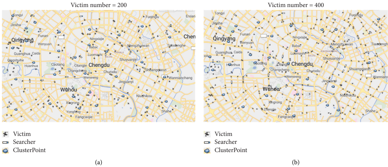
FIGURE 8: The experiment environment of the ERSCIED (200 victims (a) and 400 victims (b)).
