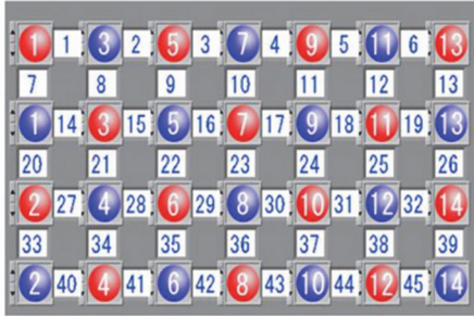
FIGURE 1: The area between 14 pairs of probes comprised 45 channels, 3 cm apart. The red color represents emission probes, and the blue color represents detector probes.
