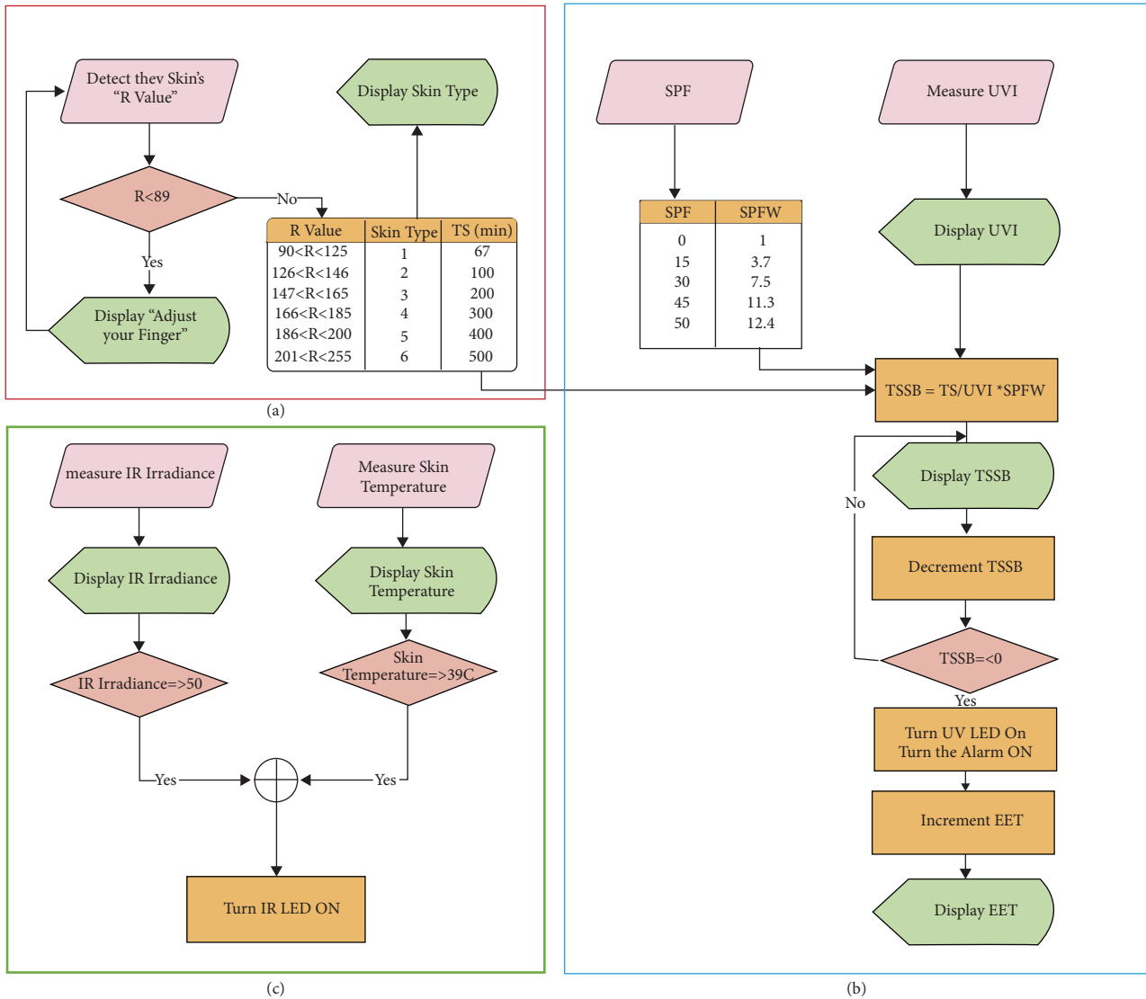
FIGURE 5: Algorithm behind the solar band. (a) Skin type classification algorithm. (b) Exposure time algorithm. (c) IR alarm algorithm. Pink blocks for input data, red for if conditions, orange for processes, and green for displaying.
