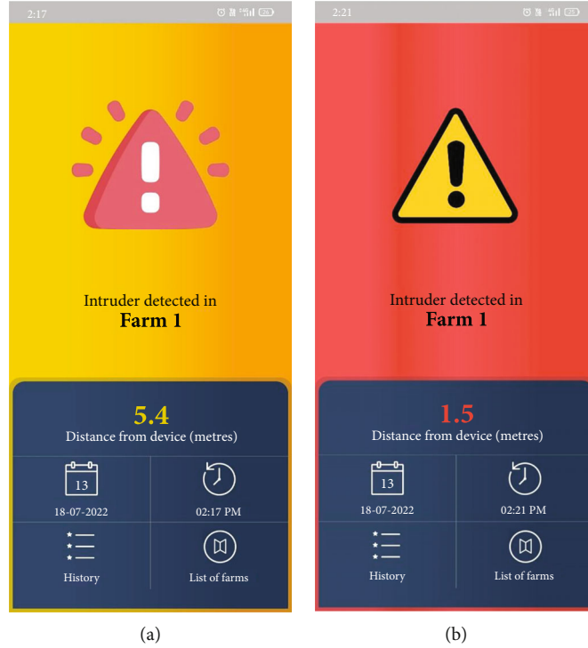
FIGURE 10: The intrusion detected at crop field store is also intimated to farm owner as an alert on an Android application that is installed on his smartphone. (a) Yellow alert: the intruder is first detected and is within 7 meters from the farm store door. (b) Red alert: the intruder continues to proceed towards the door of the farm store and is within 2 meters.
