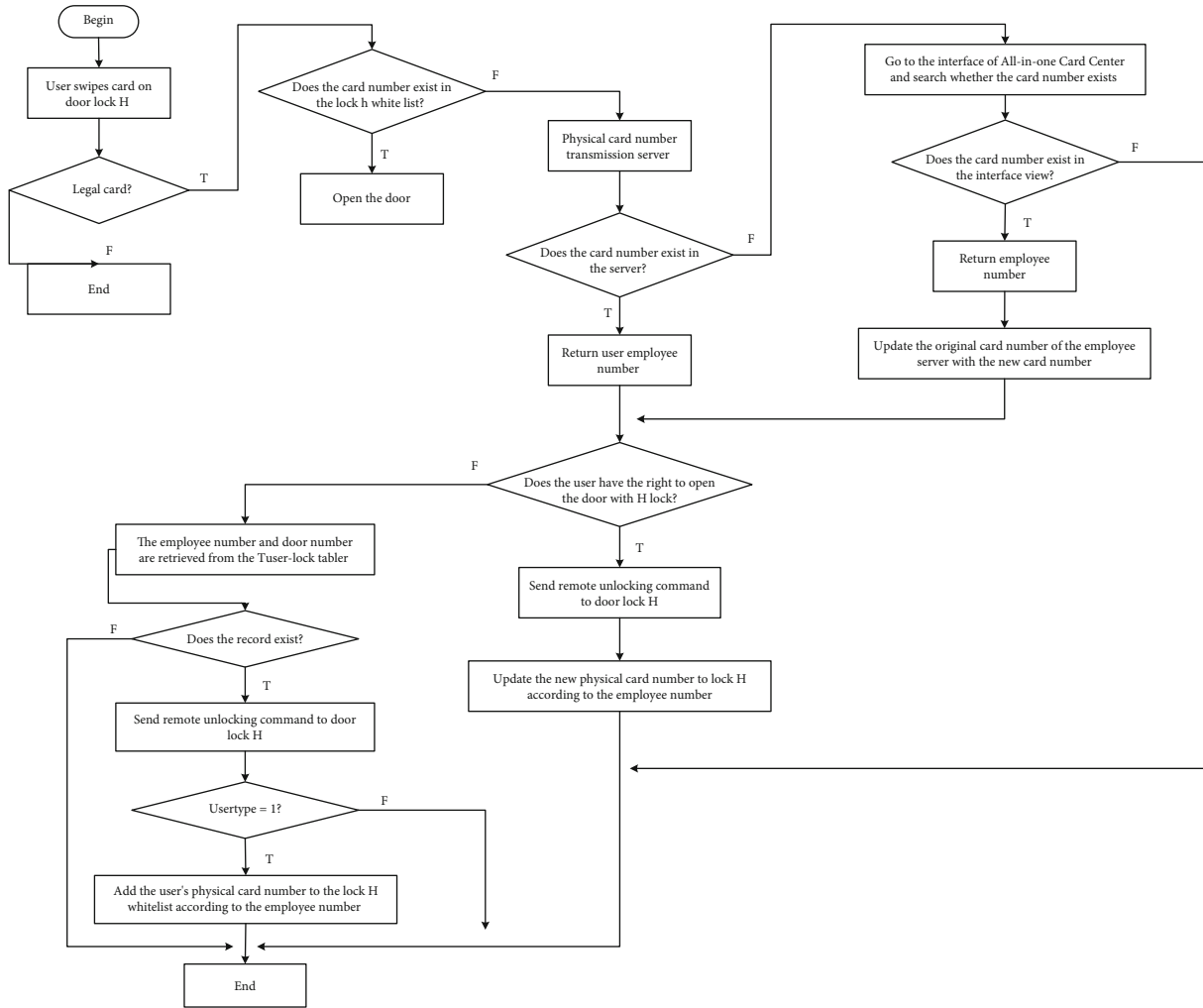
FIGURE 6: Flowchart of unlocking procedure.
