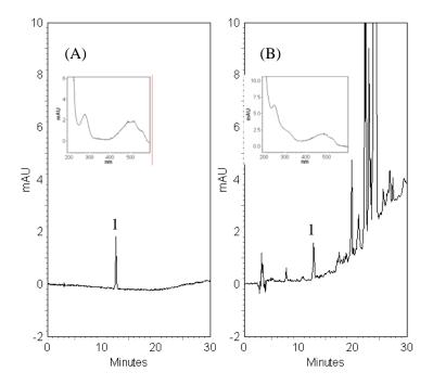
Fig.1 The content of the LR extracts as detected by HPLC chromatography. LR has an absorbance peak at 520 nm. The retention time of shikonin is 12.6 min. (A) shikonin standard. (B) ethanol extract of LR. The concentration of shikonin in the LR extract was determined to be 0.62 mg/g.
