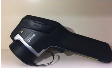
FIGURE 3: Thermal imager (E60, FLIR® Systems Inc., Wilsonville, OR, USA).
