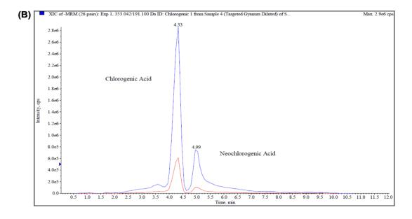
Figure S1. LC-MS/MS full chromatograms of G. procumbens (A) and chlorogenic acid (B).
