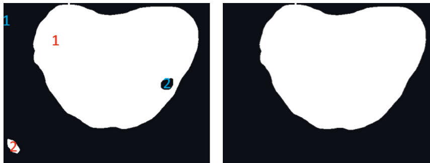
FIGURE 5: Mask morphology processing. The connected component with the largest area in black or white will be marked as “1” and other connected components will be eliminated.
