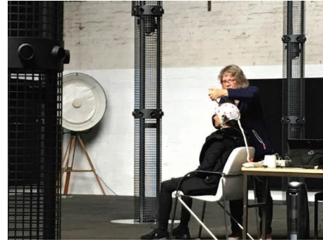
FIGURE 2: EX1 EEG measurements at MONOM center for spatial sound Berlin. The omnidirectional speakers are placed in the observed black columns. Each column holds 3 speakers: at ground level, top (4 m), and middle.
