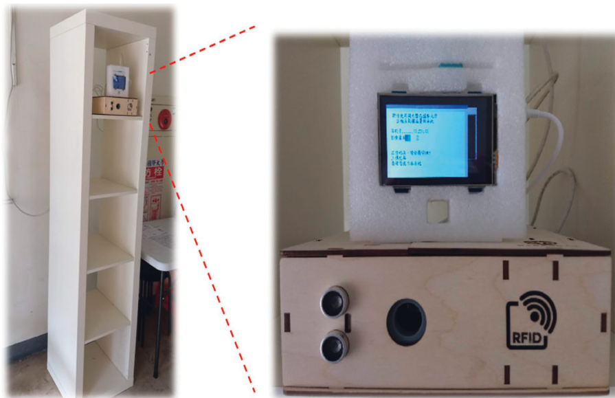
FIGURE 11: Station set up in the lobby of a student dormitory. The small LCD screen (left part) acts as an interactive user interface.
