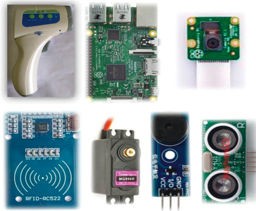
FIGURE 2: Components of the autothermometer system (from top left): a forehead thermometer, a Raspberry Pi device, a camera module, an RFID reader, a servo motor, a buzzer, and an ultrasonic module.
