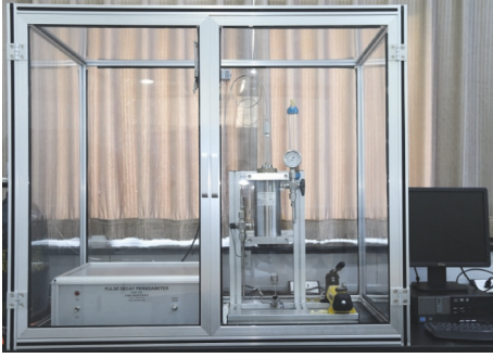
FIGURE 3: Setup to measure permeability of tight rock through pressure-pulse-decay method.
