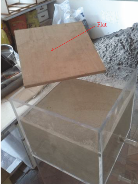
FIGURE 2: Soil being filled into the tank model. Every 5 cm depth soil layer is pressed by the flat.
