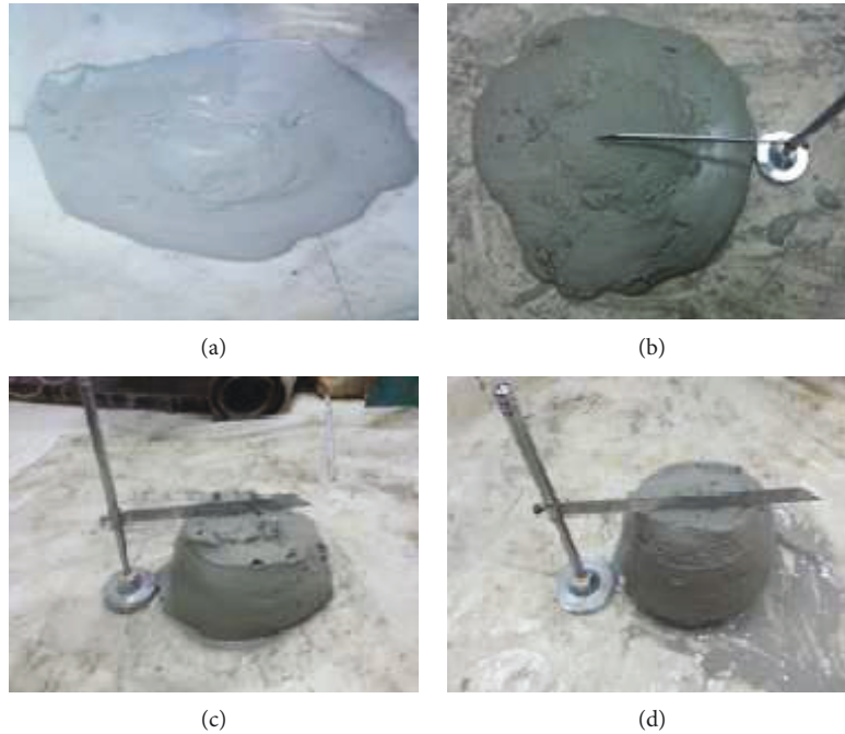
FIGURE 9: Results of slump tests at mass fractions of (a) 65%, (b) 68%, (c) 70%, and (d) 72%.
