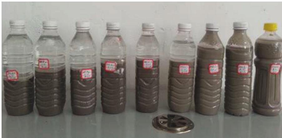
FIGURE 7: Bleeding water of PGBS in the bottles.
