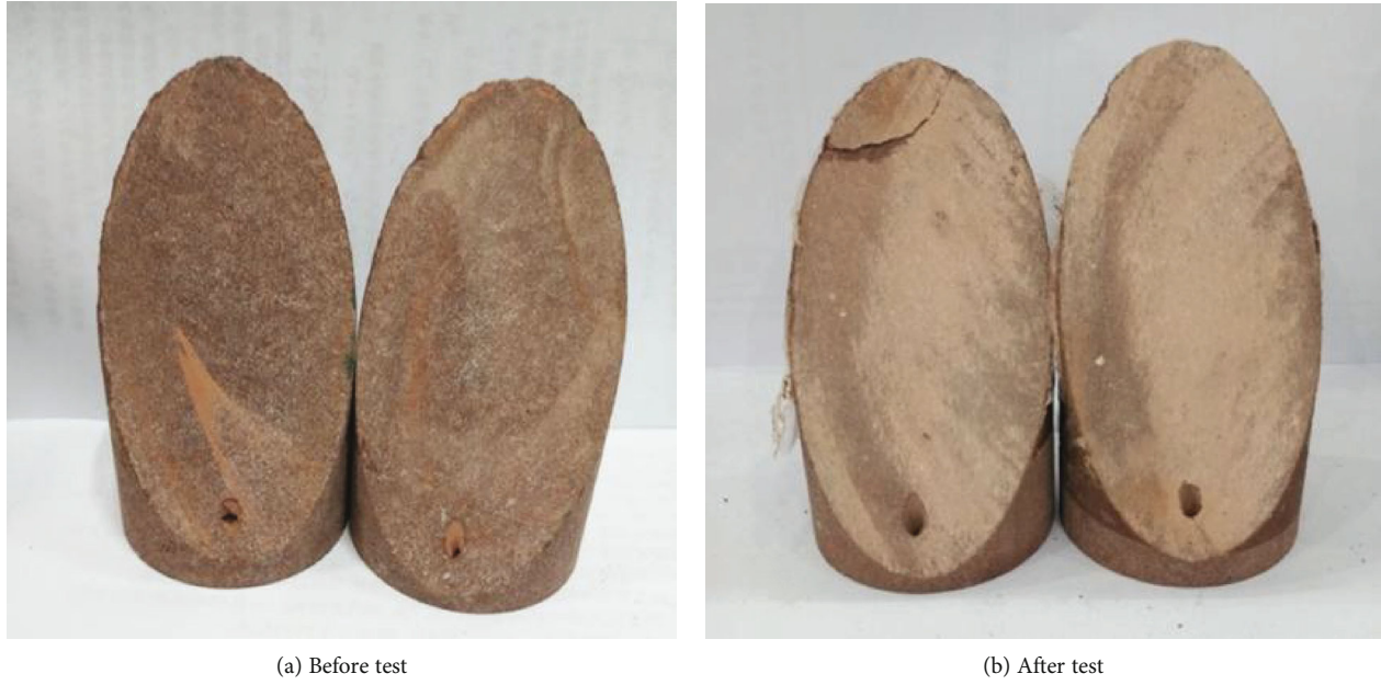
FIGURE 6: Comparison of untested fracture surfaces and tested fracture surfaces of SC-5.
