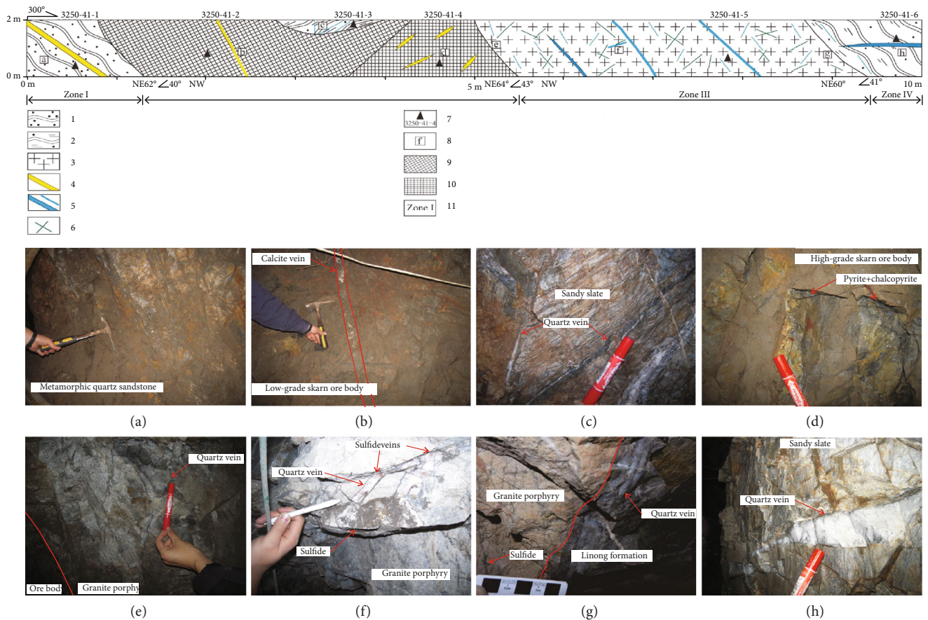
FIGURE 5: The sketch map of 41#-1 mining stope at a 3250 m level in the YCD, Yunnan, China. 1-quartzite, 2-sericite slate, 3-MGP, 4-calcite veins, 5-quartz veins, 6-sulfide veins, 7-sample and numbers, 8-photos, 9-low-grade SOB, 10-High-grade SOB, 11-mineralization-alteration zone. (a) The strongly silicified quartzite, which developed the veins, scattered, and disseminated pyrite. (b) The low-grade SOB, which developed disseminated pyrite and chalcopyrite and later calcite vein. (c) The sericite slate, which developed partially disseminated pyrite and later calcite vein. (d) The high-grade SOB and developed disseminated pyrite and chalcopyrite. (e) The irregular contact line of the MGP and SOB, which developed a large number of quartz veins in the MGP. (f) The MGP, which developed vein-disseminated metal sulfides (pyrite, chalcopyrite, bornite, and molybdenite) and quartz veins. (g) The irregular contact line of the MGP and sericite slate, which developed veins metal sulfides in the MGP, and there are many quartz veins in the sericite slate of Linong formation. (h) The sericite slate, which developed the later quartz veins, disseminated-fine vein metal sulfides. Zone I: carbonatation, silicification, argillization, sericitization, and weak pyritization. Zone II: skarnization, pyritization, chalcopyritization, silicification, and carbonatation. Zone III: the mineralized granite porphyry dike with strong silicification, as well as calcitization, pyritization, chalcopyritization, molybdenitization, sericitization, and chloritization. Zone IV: silicification, pyritization, sericitization, and chloritization.
