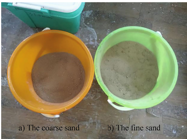
FIGURE 12: Prepared silty fine sand and medium-coarse sand.
