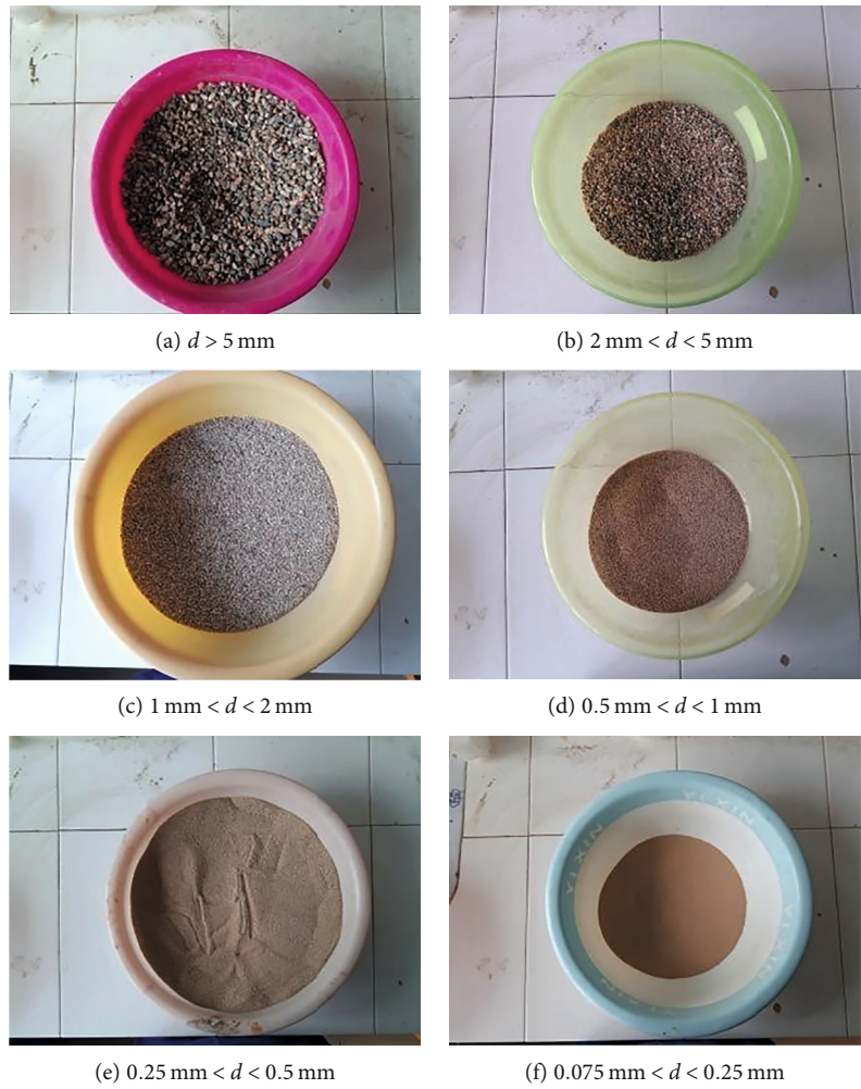
FIGURE 11: Screened soil with different particle sizes.
