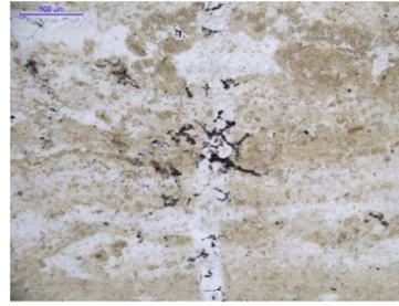
G115 mainly consists of algal dolomite and a small amount of micrite dolomite, develops fractures, dissolution pores and intercrystalline pores
