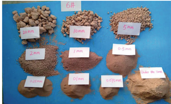
FIGURE 14: The screening test results of soil-rock mixture sample 6#.
