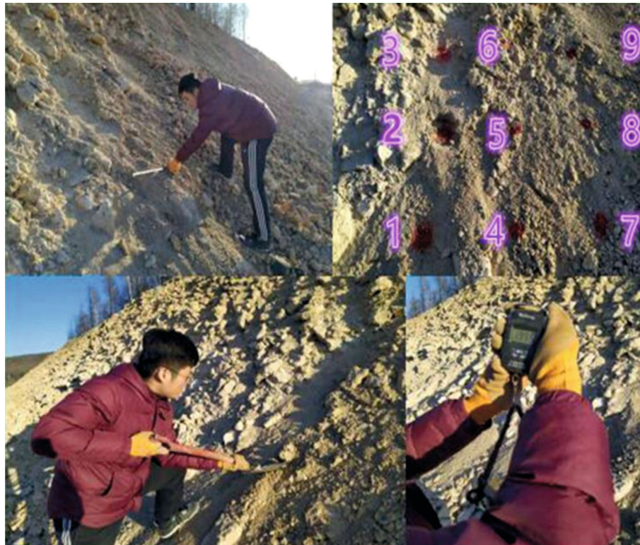
FIGURE 13: The soil-rock mixture sampling process.
