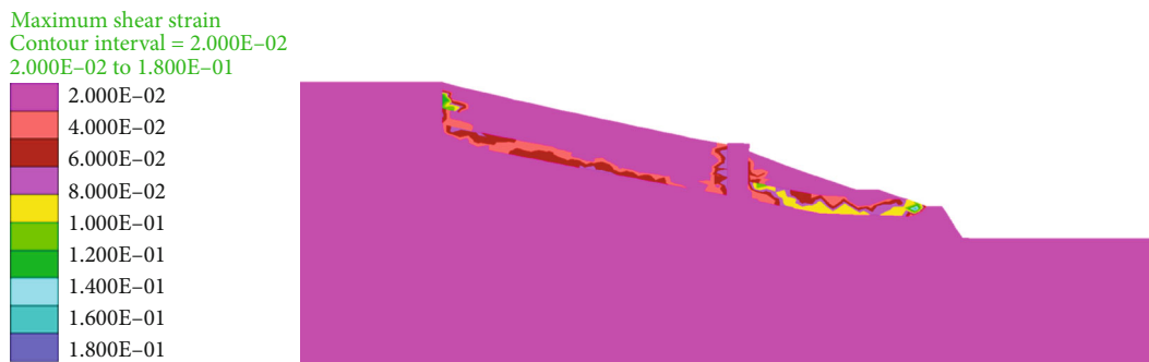
FIGURE 8: Shear strain contours.
