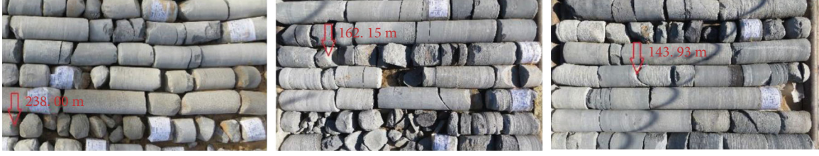
FIGURE 4: Drill-core photographs of JE1 borehole: (a) RQD is zero of CZ; (b) first fresh vertical fracture and smaller RQD of TFZ; (c) initial high angle fracture and larger RQD of NFZ.
