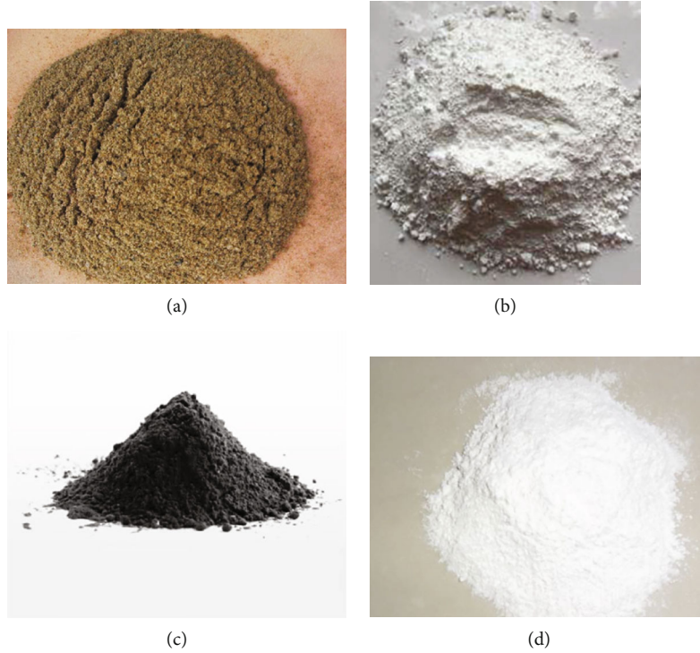
FIGURE 1: Raw materials of the similar material: (a) river sand, (b) barite powder, (c) cement, and (d) gypsum.
